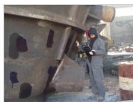
Pot 두께검사 UT Checking thickness of Pots
